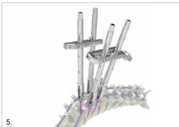
**NOTE:** Use the Key for the derotation clamp and also the Handle to tighten the Derotation Clamp with the derotation tube.
