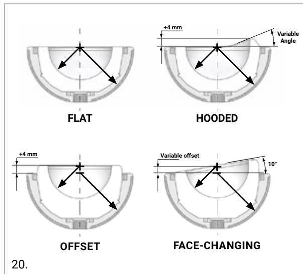
For the hooded liners, the hood makes an angle which is size dependant:
