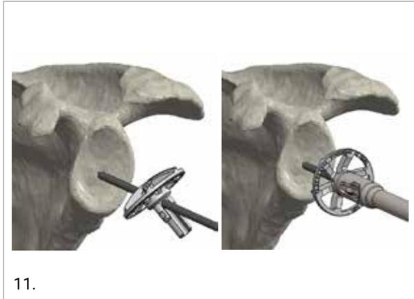
By visually checking the size of the reamer, the final evaluation of the size of the Baseplate to be implanted can be made.
