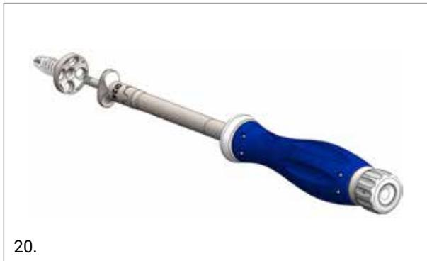
Secure the Baseplate to the impactor by screwing the rod until fixed.
