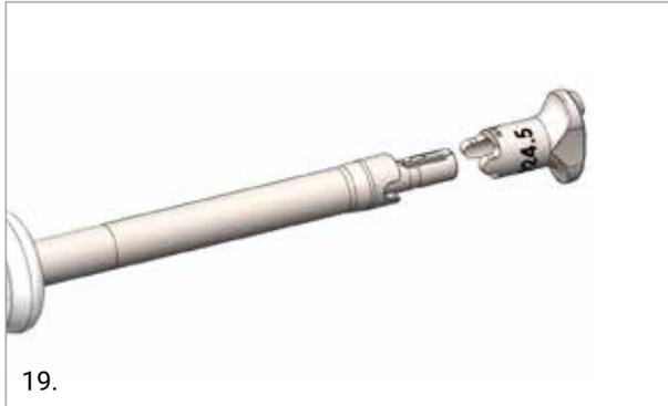
Slide the M5 Fixation Rod into the assembled Baseplate impactor.
