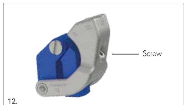
Assemble the stem repositioner by unscrewing the screw with the 3.5mm screwdriver to open the plastic clamps. Then, assemble it to the implanted stem until this is firmly seated between the plastic clamps and re-tighten the screw. The metal body should be positioned on the medial side of the stem.
