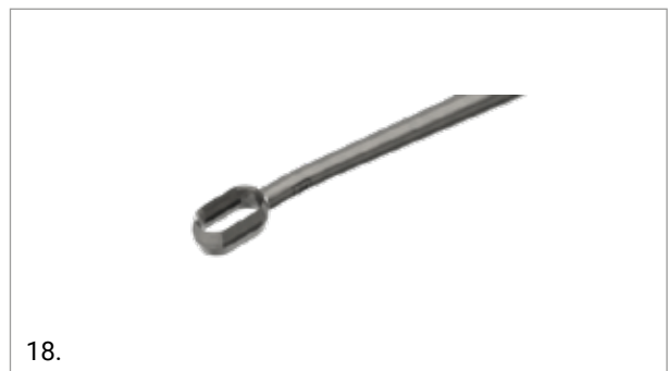
Curette 10° Small (Ref. 05.11.10.0013) Bent tip 10°, sharp on both sides, size small (Ø4mm), WL 180mm
