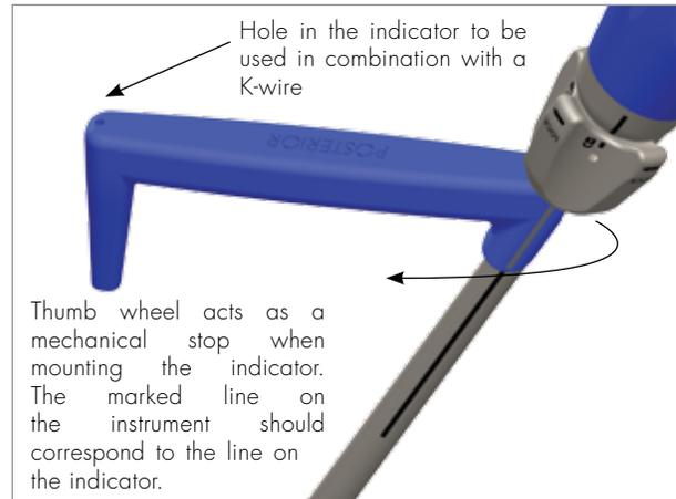
The tip of the implant position indicator will point at the spinous process and center of the implant, when the 60° angle is set.
